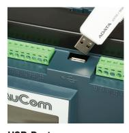
**USB** Port The new USB port allows straightforward upload, download and storage of starter performance information, increasing your ability to manage the system effectively.
